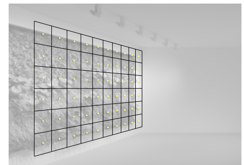
Light calculation for uniformity of the illuminance of a green wall by means of a measuring plane for vertical illuminance
